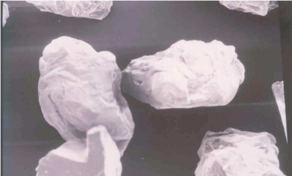
Fig. 3. Scanning electron microscopy micrograph of filter sand used in Orangedale field investigation.
