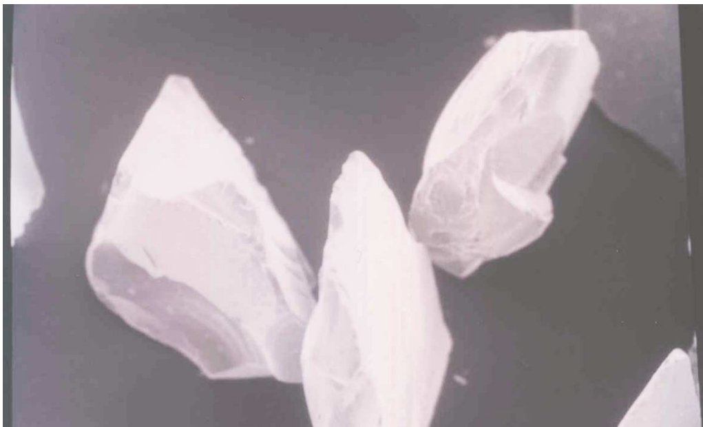
Fig. 4. Scanning electron microscopy micrograph of crushed glass used in Orangedale field investigation.
