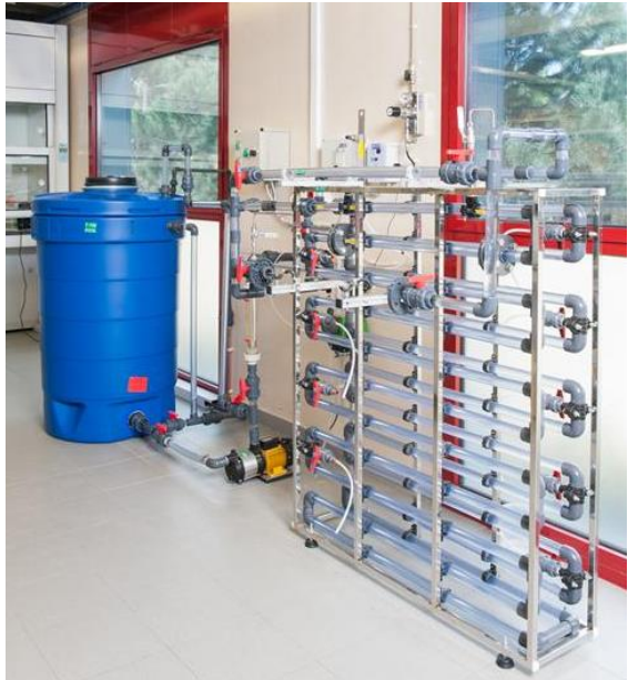
Halia ® pH neutralisation system pilot plant at Bellaterra (Barcelona - Spain)
